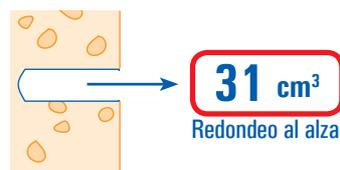
$$\text{VOLUMEN (cm}^3\text{)}_{\text{VARILLA}} = \frac{3.1416 \times 1.2 \times 1.2 \times 20}{4} = 22.62 \text{ cm}^3$$
